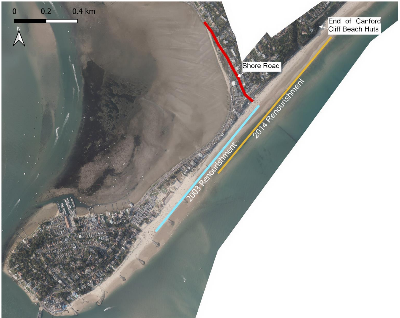
Figure 7 Overview of features at Sandbanks, including the extent of two renourishment schemes in 2003 and 2014.
