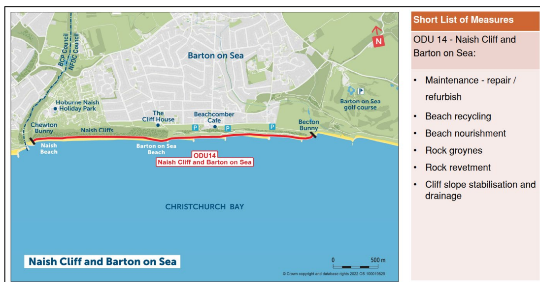
Example of short-list measures for Naish Cliff and Barton on Sea (Source: BCP Council).
