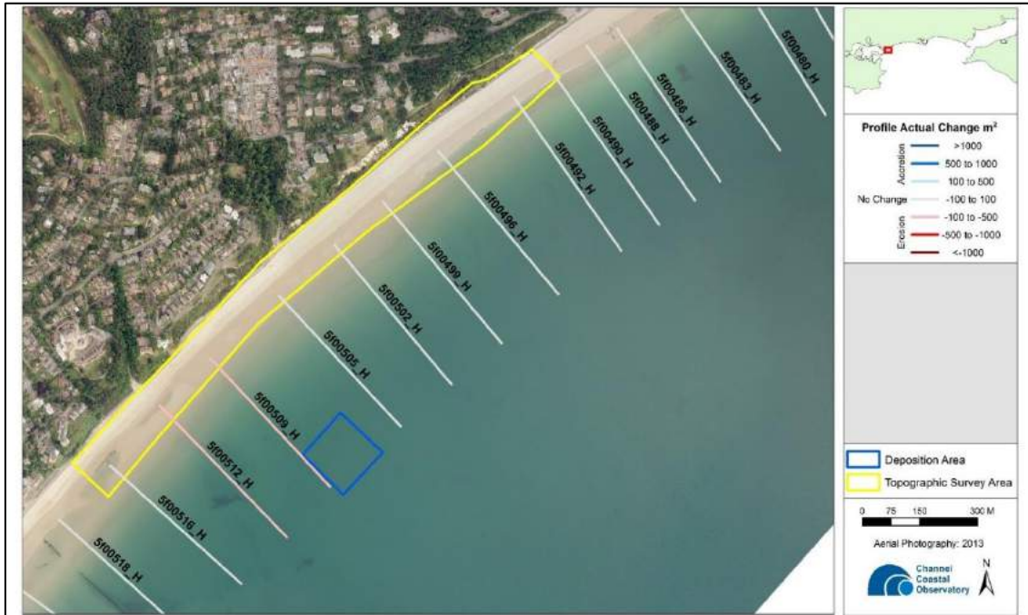
Figure B.7 Longer term change in bathymetry cross-sectional area in the trial area from May 2006 to May 2014
