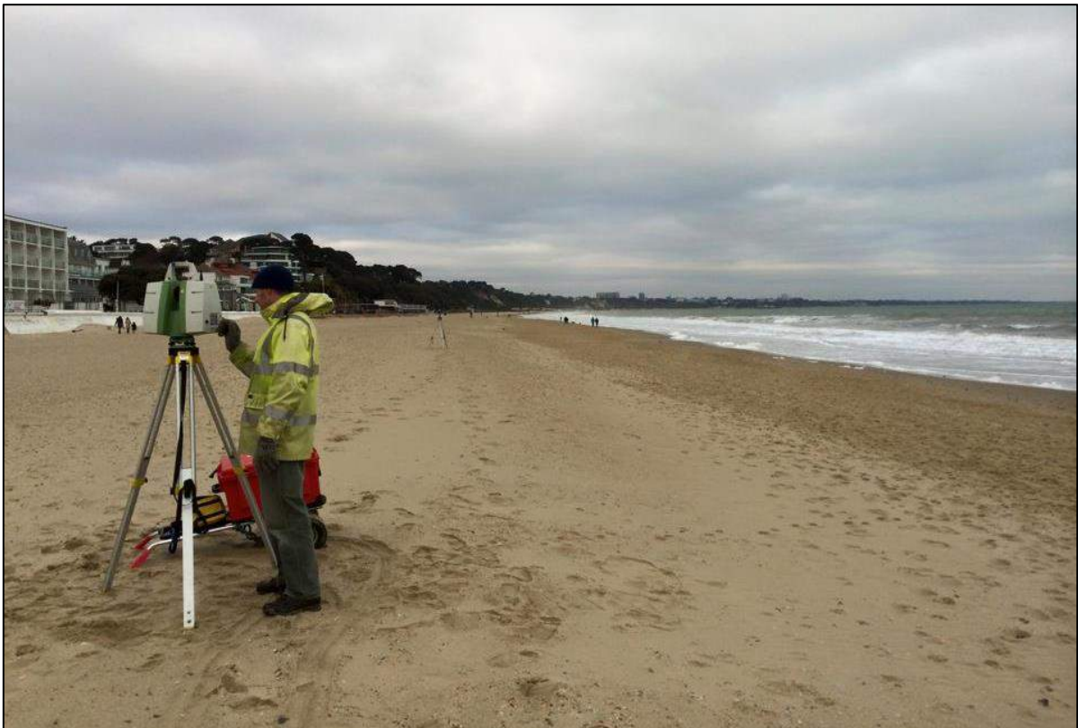
Figure A.1 Using a laser scanner on Poole beach
